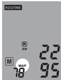
❖ *The Mean Arterial Pressure MAP in this device is determined from the maximum peak of the oscillometric envelope curve.*
