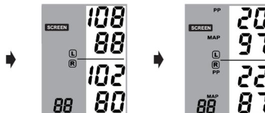
※ When the measurements are completed, the blood pressure measurement corresponding with the consistently higher arm will blink continuously for 5 seconds. If no significant difference (20 mmHg for systolic and/or 10 mmHg for diastolic blood pressure) exists between the two arms, neither measurement will blink.
